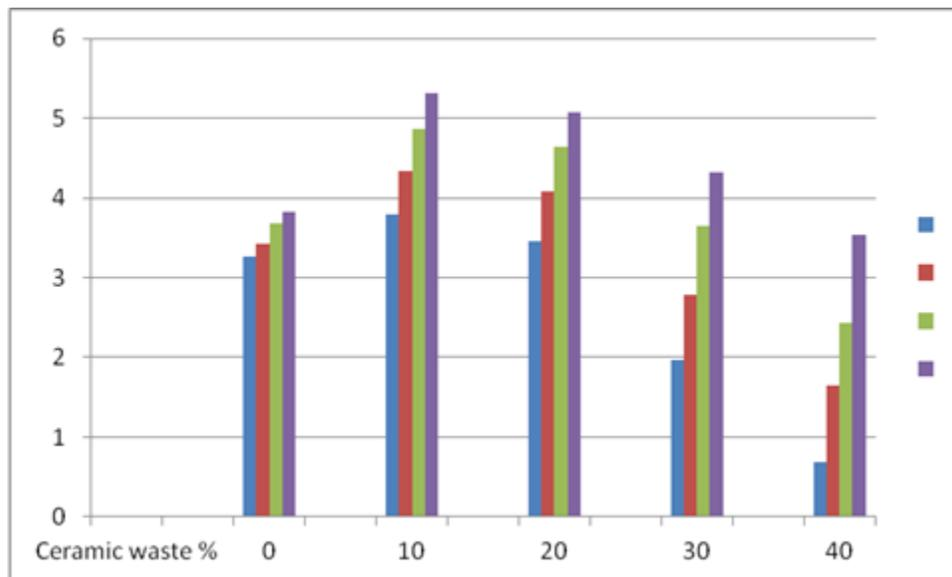
Fig. 6: Flexural strength graph with varying percentages of ceramic waste for 7, 28, 56 and 90 days
