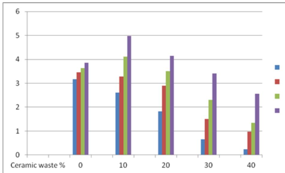
Fig. 4: Split tensile strength graph with varying percentages of ceramic waste for 7, 28, 56 and 90 days
