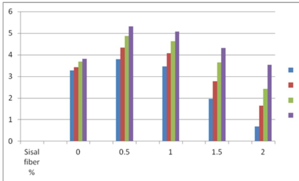
Fig. 5: Flexural strength graph with varying percentages of sisal fiber for 7, 28, 56 and 90 days
