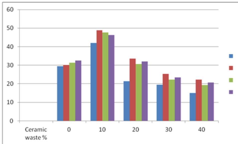
Fig. 2: Compression strength graph with varying percentages of ceramic waste for 7, 28, 56 and 90 days
