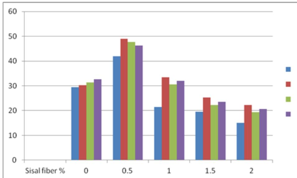
Fig. 1: Compressive strength graph with varying percentages of sisal fibers for 7, 28, 56 and 90 days
