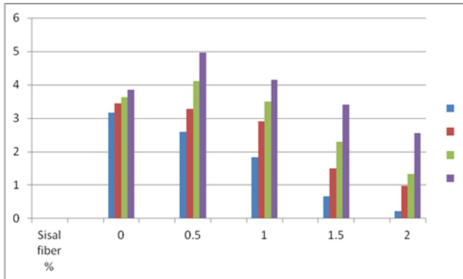
Fig. 3: Split tensile strength graph with varying percentages of sisal fibers for 7, 28, 56 and 90 days
