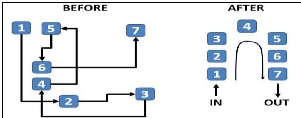
One piece flow is a condition that exists when products move through a manufacturing process one unit at a time, at a rate determined by the needs of the customer. The opposite of one piece flow is mass production with batches and queues. One piece flow focuses on flow efficiency rather than on resource efficiency.
