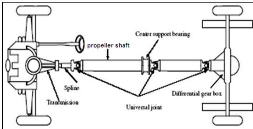
Fig. 3: Conventional two-piece propeller shaft arrangements for rear wheel vehicle driving system
