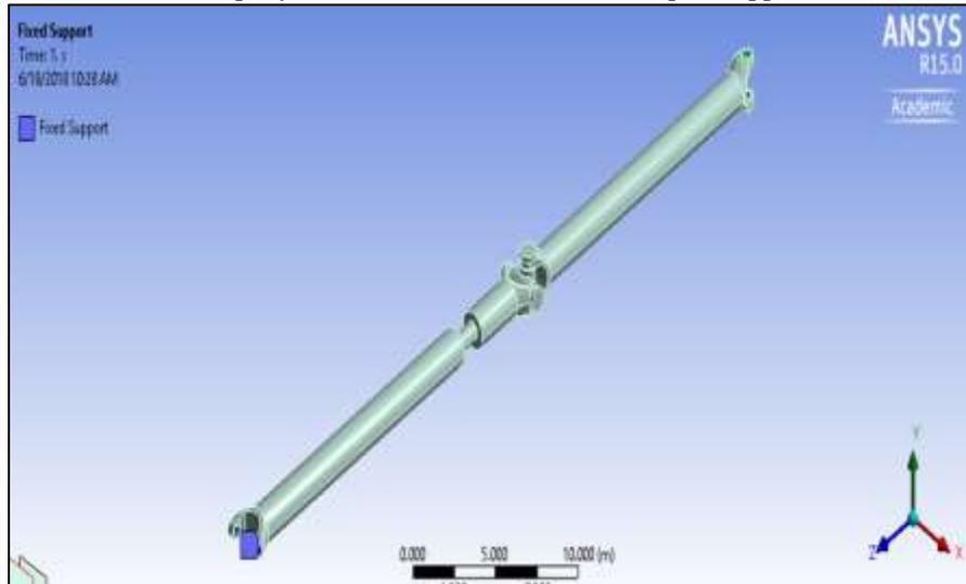
Fig. 7: Finite element model of Hm Carbon/Epoxy shaft
