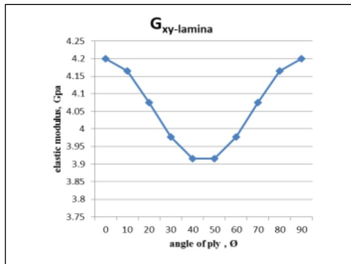
Fig. 6: The variation of the  $G_{xy\text{lamina}}$  with ply orientation for HS Carbon/Epoxy
