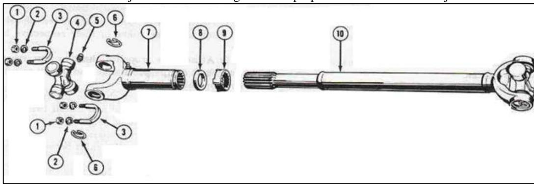
Fig. 4: Parts of Propeller shaft and universal joint
