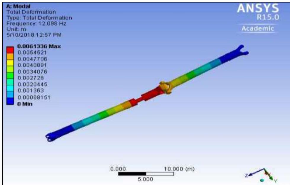
Fig. 15: mode shape of a Hm carbon propeller shaft
