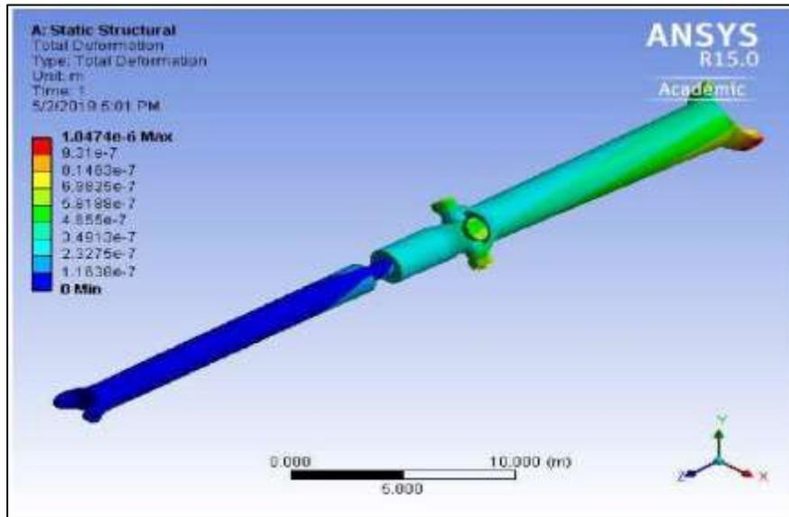
Fig. 13: Total deformation of a conventional steel propeller shaft
