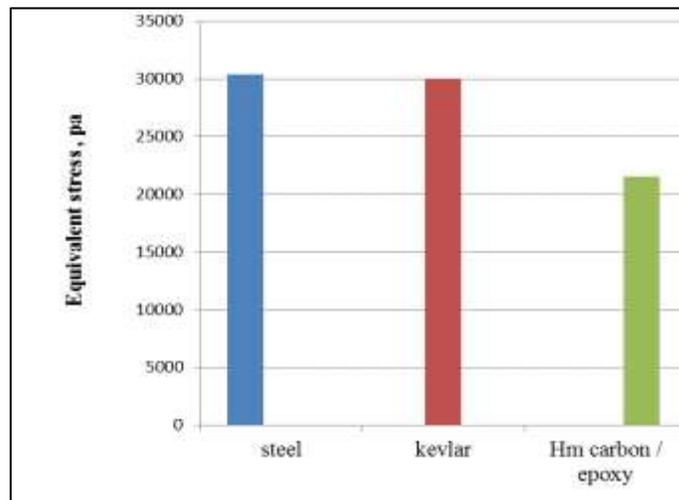
Fig. 12: Von- mises stresses for our proposed materials at a particular load
