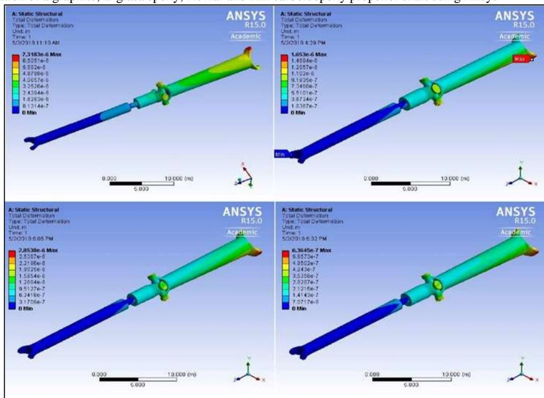
Fig. 14: Total deformation of a Propeller shaft with our proposed material
