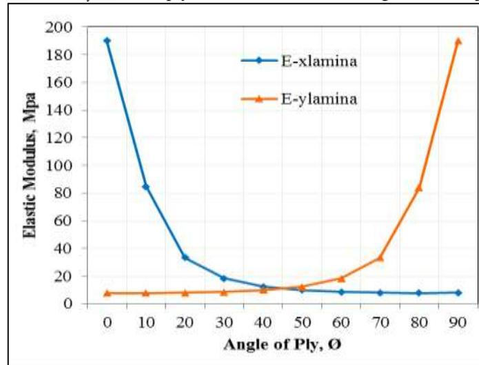
Fig. 5: The variation of the  $E_{x\text{lamina}}$  and  $E_{y\text{lamina}}$  with ply orientation for Hm Carbon/Epoxy
