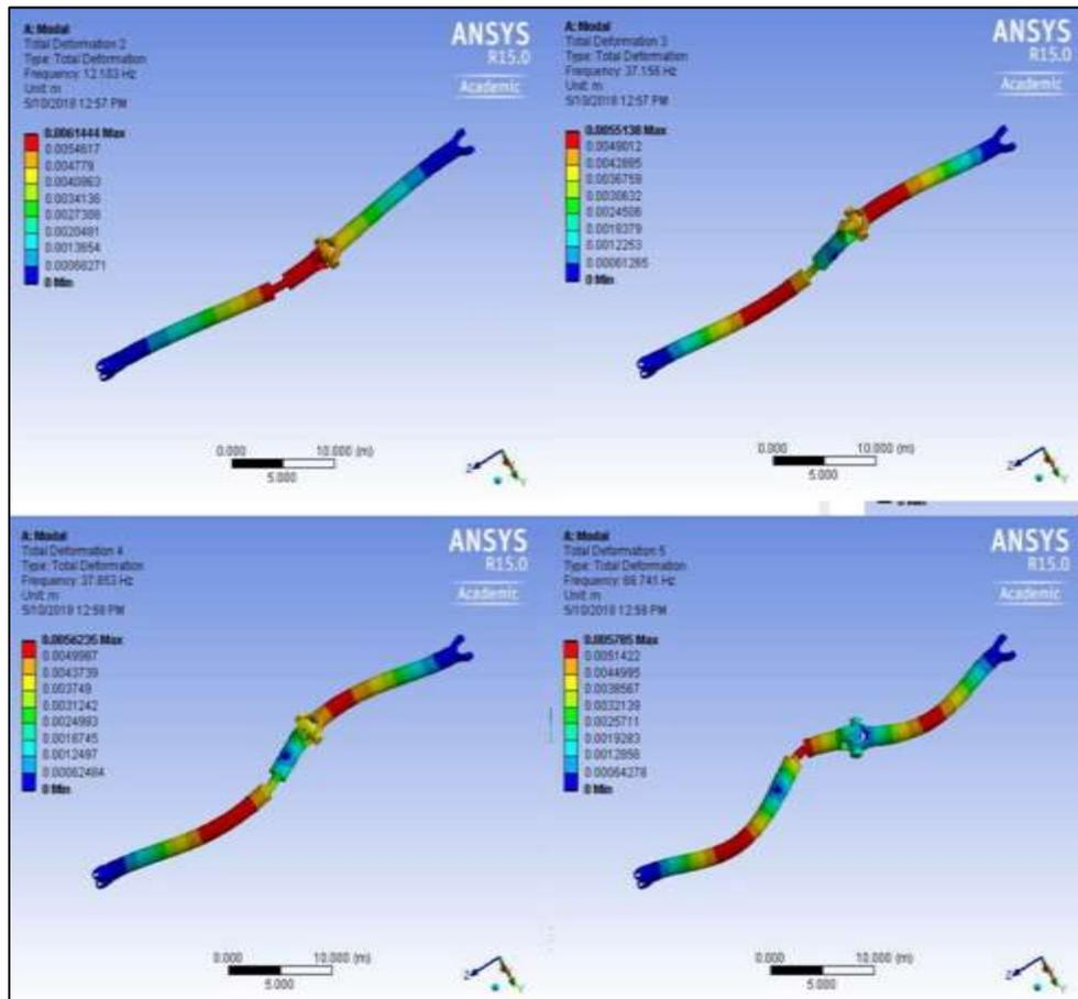
Fig. 16: Different mode shapes of Hm carbon/Epoxy propeller shaft
