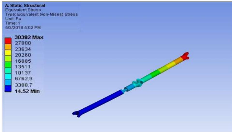
Fig. 9: Equivalent stresses of a steel propeller shaft
