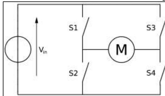
Fig. 4: H bridge circuit diagram
