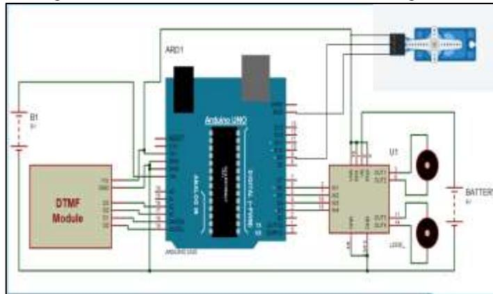
Fig. 3: Circuit diagram of DTMF controlled tractor
