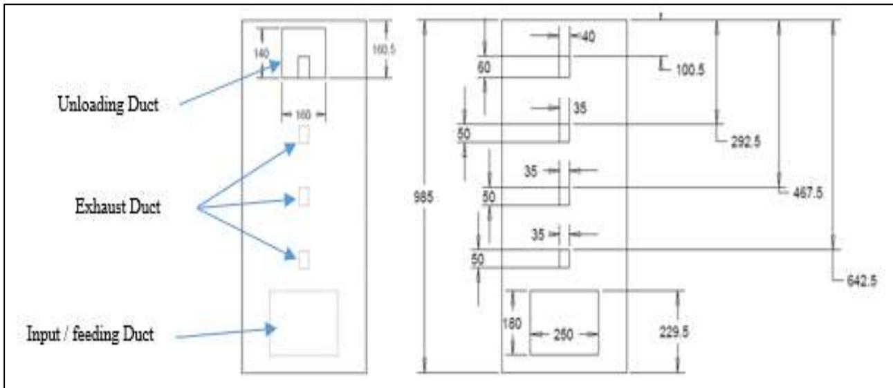
Fig. 4: Outer Shell Cad Drawing
