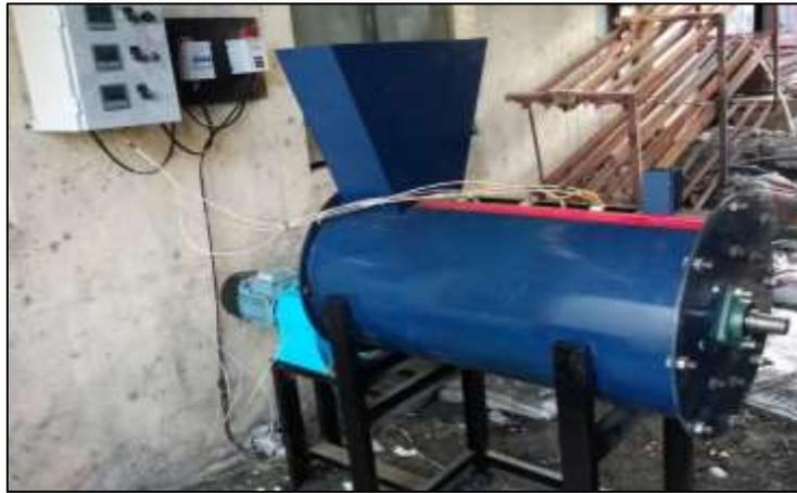
Fig. 5: Fully Constructed Electrical Coal Dryer
