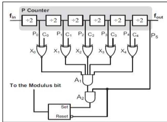
Fig. 8: Integrated P&S counter
