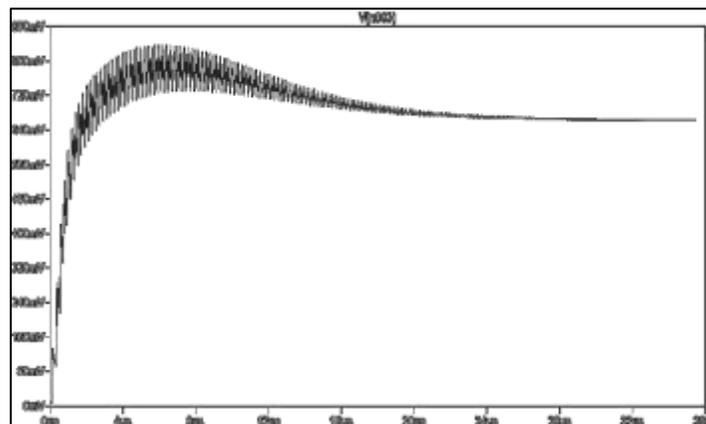
Fig. 10: Vcntr for VCO for c4c3c2c1c0=00001
