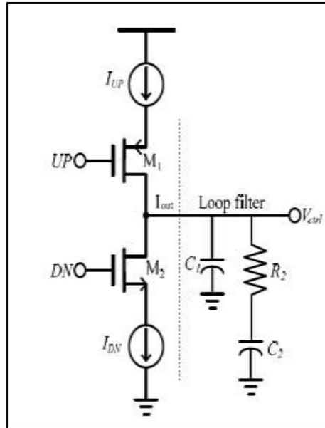
Fig. 4: Charge pump with loop filter
