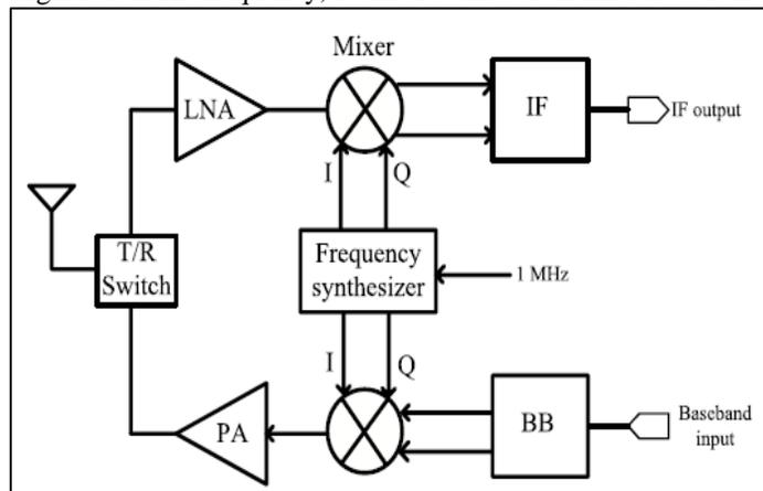
Fig. 1: The role of frequency synthesizer in a transceiver
