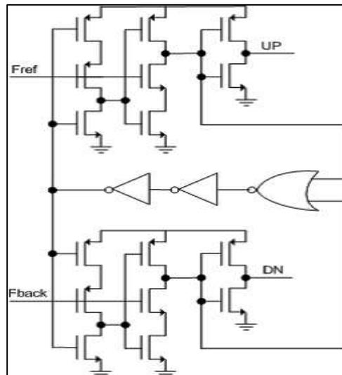
Fig. 3: Phase Detector
