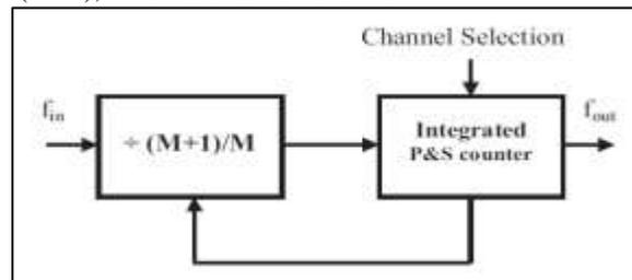
Fig. 6: Asynchronous programmable modulo-P counter
