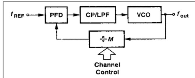
Fig. 2: Block diagram of frequency synthesizer
