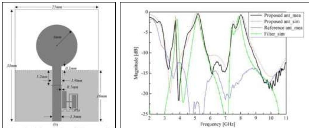
Fig. 2: Proposed Filtenna with triple notch characteristics [2] and its Return Loss
