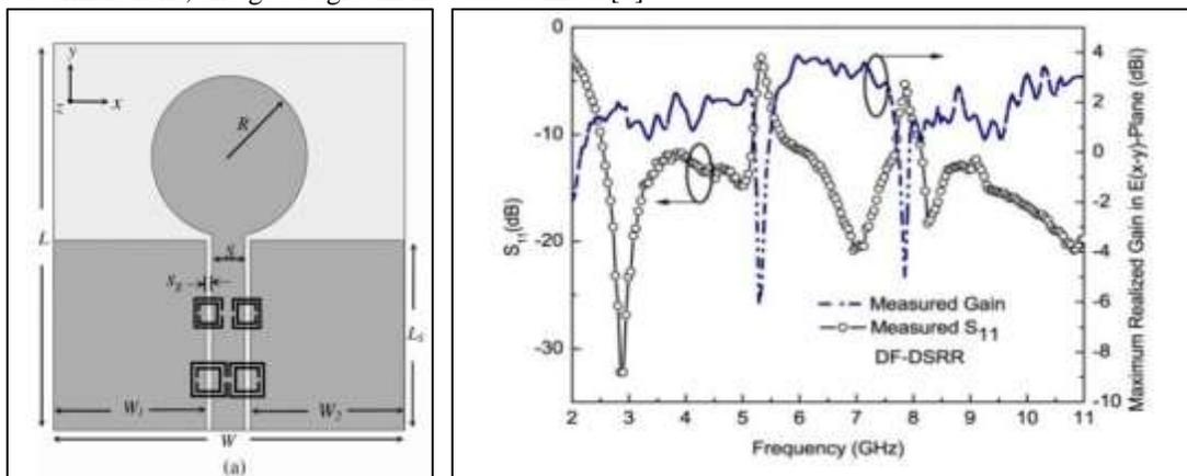
Fig. 4: Proposed Filtenna with dual notch characteristics using SRR [4] and its measured Gain & Return loss
