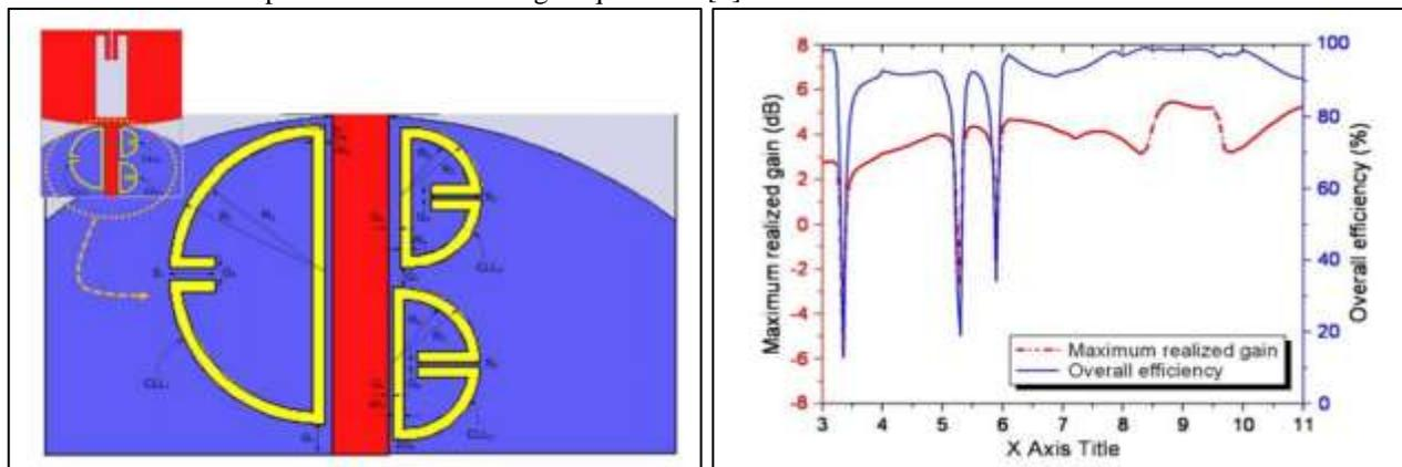
Fig. 3: Filtenna with triple notch characteristics achieved using CLL resonators [3] and its Gain
