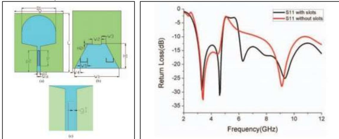
Fig. 5: Proposed Filtenna with notch characteristics [6] and its measured Return loss
