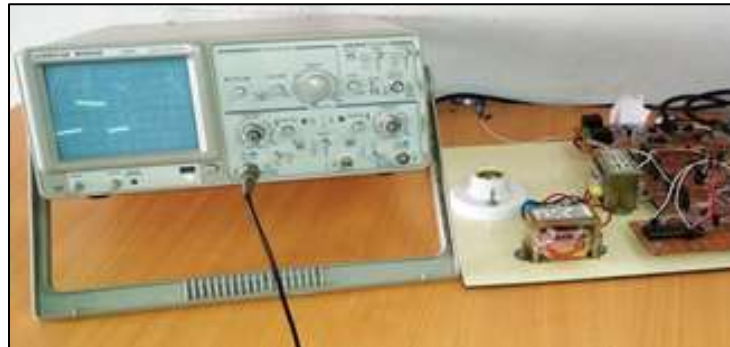
Fig. 8: Obtained Square Wave Output from Pin RB1 of PIC16f877A
