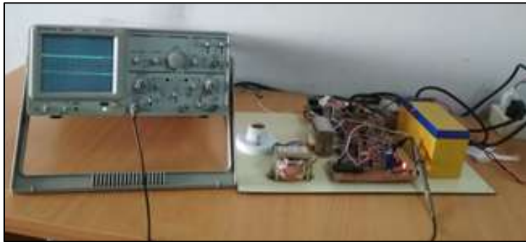
Fig. 10: Obtained SPWM Output from Pin RC1 of PIC16f877A
