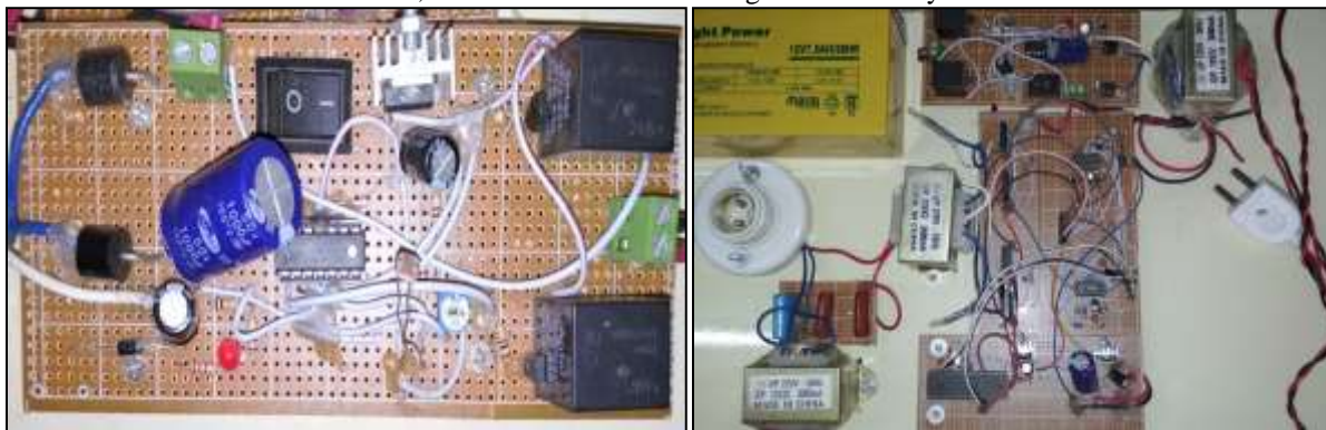
Fig. 4: (a) Sine wave Inverter Circuit Overview (b) Dark down and Power Circuit Overview.
