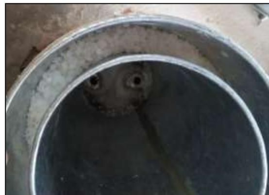
Fig. 3: Paraffin Wax filled in Annulus as Phase Change Material
