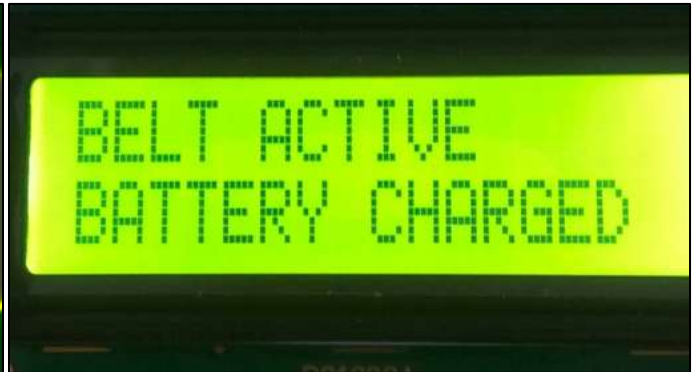
Fig. 4.6: Belt (Active) and Battery Status
