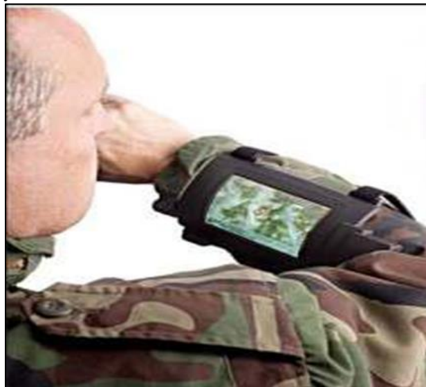
Fig. 1: Demonstration of a prototype wrist unit that is worn by soldier with a navigation display on
